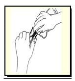
Push the blue port adaptor fully into the white gripper.
